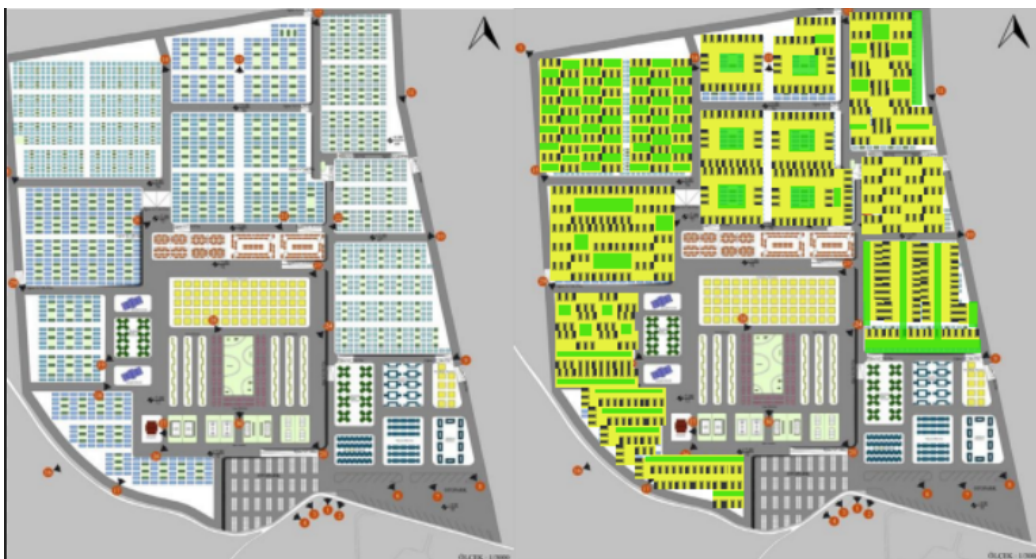
Figure 7: On the left, the container city prepared by Dayanır et al. (2022) for İzmir-Seferihisar, taking into account its compliance with the regulations; on the right, the expression of the remaining common areas in yellow and green when the containers are worked in 3 floors with black spots (Prepared by the authors).
