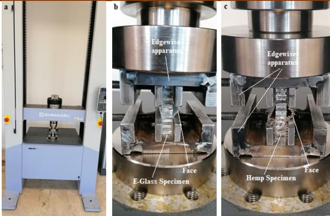
Figure 3. Edgewise compressive tests of test device (a), E-Glass (b) and Hemp (c) sandwich specimens
